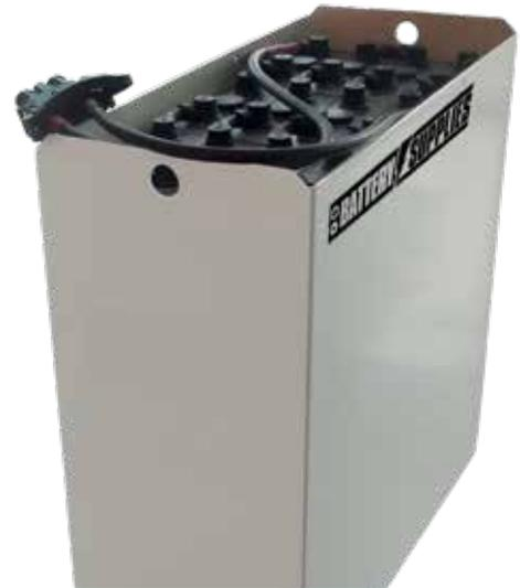
**Attention:** the charger must be adapted to gel PzV charging profile. We recommend 12h charging. For 8 hours charging, the capacity should not exceed 600-650 Ah for 24V, 350 Ah for 48V or 200 Ah for 80V batteries.
