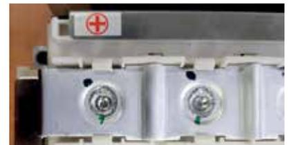
In industrial and logistics applications only LiFePO4 is used. It is important to understand that this technology does not ignite or explode, even if the battery breaks down. It is fully protected. The cells are assembled in modules with laserwelded busbars. This connection reduces the internal resistance and reduces the risk of poor connections.
