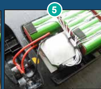
Placement du nouveau BMS (Battery Management System)
