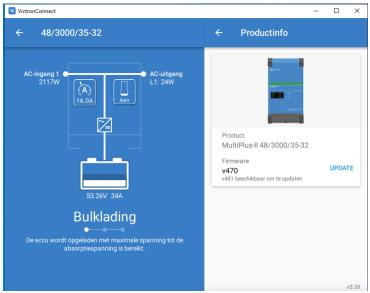
After the three devices have the latest firmware, the VictronConnect program can be closed and all Mod -bus cables between the different Multipluses can be reconnected.
