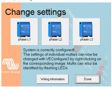
Now repeat the above steps for the second and third inverter. Then close the program via "Done". All operating parameters are now in the devices and the connection via the interface can be disconnected with the PC.
